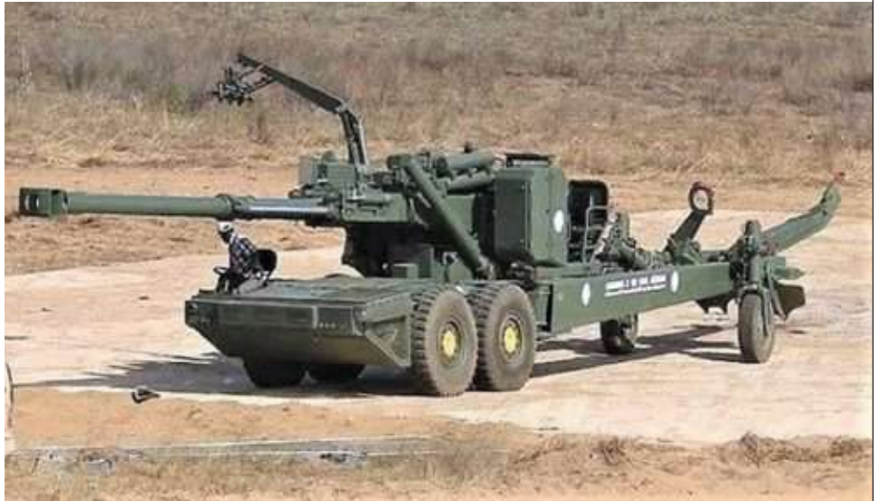
Trials of the 155mm 52 calibre Advanced Towed Artillery Gun System have been completed
